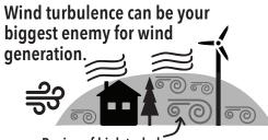
Turbulence is created by surrounding obstacles. These obstacles severely reduce the amount of power you can generate and put a lot of wear and tear on your equipment.
